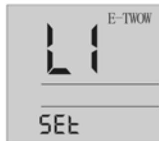
b. Move to menu with button [ LIGHT] L1-L2-L3-L4-L5
